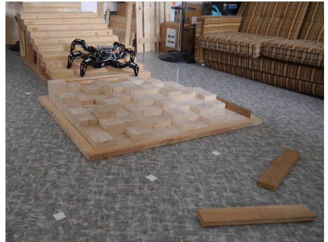
Figure 6: Testing scenario consisting of small obstacles (bottom right corner) on the office floor, followed by a pool of wooden blocks and ending with climbing the stairs.
