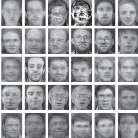
**Fig. 8.** Reconstructed images for GD-CLS NMF method ( $k = 100$ ), examples of bad reconstruction were included.
